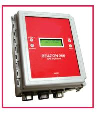
The Beacon<sup>™</sup> Series is housed in a NEMA 4X rated case for a weather tight seal. This case design complies with the new lock out / tag out standard and can be fully secured. An external reset switch allows the alarm to be silenced from outside of the controller housing. The Beacon<sup>™</sup> units ship complete with a wall mounting kit for easy installation.
