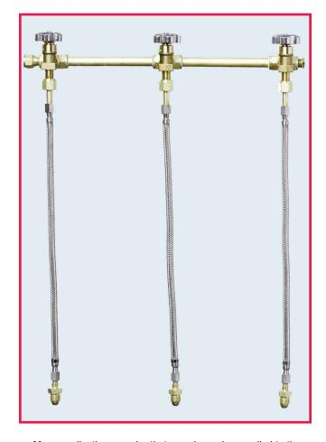
Many applications require that gas always be supplied to the process and the flow can not be shut down to replace empty cylinders or must feed gas for long periods when the system is unattended, i.e. helium to a gas chromatography laboratory. In these instances a changeover manifold is the solution. Changeover manifold control sections available in this catalog (see pages 38-43, can be used with any of the multiple station manifolds or with a single pigtail on each side.
